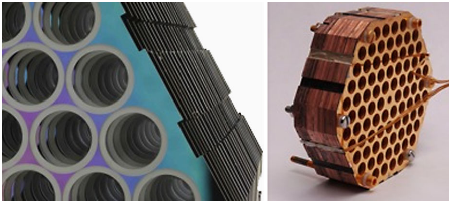
Fig. 2 (Color online) Finished platelets before final HF etch ( left ) and finished feedhorn array after plating ( right ). The finished array is \sim 55 mm wide and the wires (on right ) are used to connect the feedhorn to the cathode during plating, and are subsequently removed
