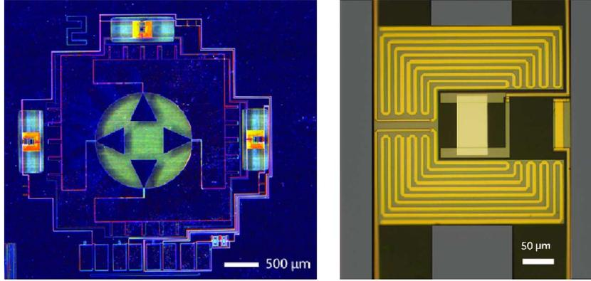
Fig. 1. (Left) Optical micrograph of the prototype polarimeter. Nb OMT fins couple X [Y] polarized light onto the isolated membranes located on the top (right side). A dark TES used for systematic error checks is located on the left. (Right) Enlargement of the thermally isolated TES island. The Al-Mn TES is located in the center. Au meander surrounds the TES, and the Au heater is located on the right.
