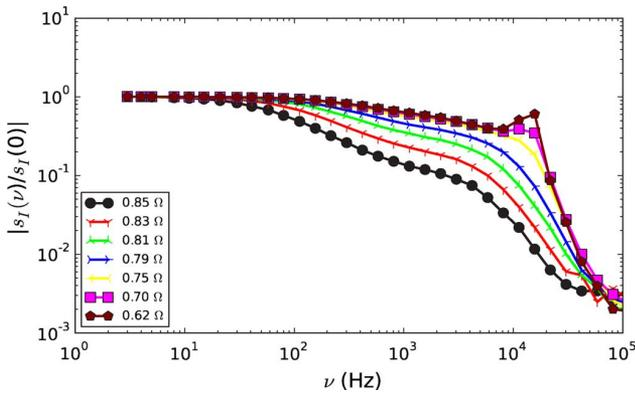
Fig. 4. Normalized responsivity measurement using the technique described in [20] for several bias points in the transition.
