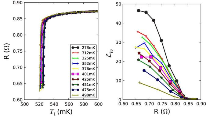
Fig. 3. Resistance versus temperature and IV loopgain ( $\mathcal{L}_{iv}$ ) versus resistance for several bath temperatures.
