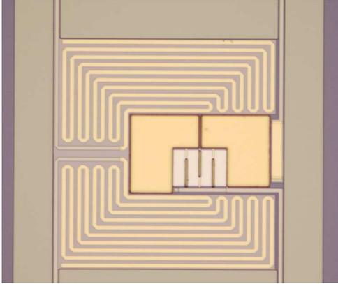
Fig. 7. Example of a second-generation TES island that includes added TES heat capacity with Au (surrounding the Al-Mn film) and lines of normal metal dots on the Al-Mn film.
