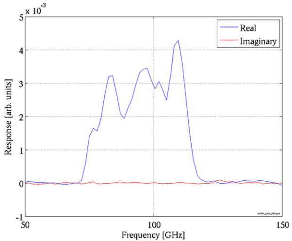
**Fig. 4** The change in Joule heating for changes in optical power incident on the detectors. The optical power is modulated by changing the temperature of a nearly black cryogenic load. The expected optical power is calculated for a Rayleigh-Jeans source assuming a 36 GHz optical bandpass (comparable to the spectra measured in Fig. 3) for which the coupling is single-moded. The measured change in Joule heating indicates an optical coupling efficiency of  $\sim 85\%$
