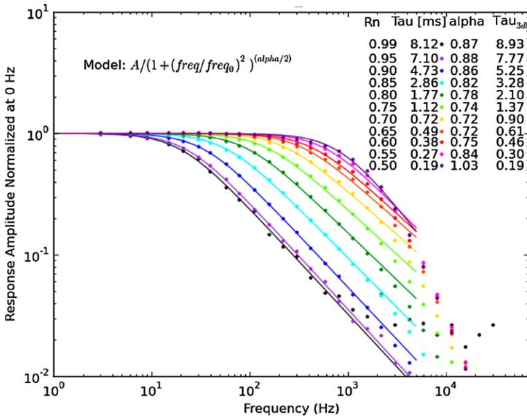
**Fig. 5** (Color online) The thermal response [1] of an ANL/KICP bolometer at various depths in the transition. At an operating depth of 0.69Rn, the detector has a thermal time constant of 0.9 ms corresponding to an electro-thermal gain of ~9 and exhibits no signs of thermal instability
