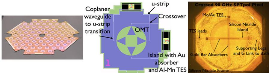
**Fig. 2** Layout for detectors that will be used for SPTpol. The images on the *left* show a 150 GHz array and a schematic of a 150 GHz array pixel being fabricated at NIST. On the *right* is an image of a crossed 90 GHz pixel fabricated at Argonne National Laboratory
