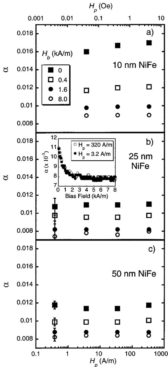
FIG. 2. Dependence of the Gilbert phenomenological damping parameter  $\alpha$  with pulse amplitude  $H_p$  at 0, 0.4, 1.6, and 8.0 kA/m (0, 5, 20, and 100 Oe) longitudinal bias fields  $H_b$ , shown for 10, 25, and 50 nm films in (a)–(c), respectively. The error bars are no larger than the size of the data points unless shown. The inset of (b) is a plot of the damping vs  $H_b$  for 320 and 3.2 A/m (4 and 0.04 Oe) pulse fields for the 25 nm thick film.
