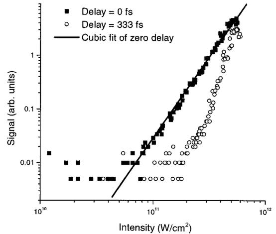
Fig. 3. DFWM FROG signal at zero time delay with a cubic fit. At a time delay of 333 fs, there is no temporal overlap of the fixed and delayed beams. The only signal arises from self-phase modulation of the beam.
