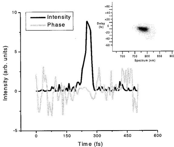
Fig. 4. FROG trace of a near-transform-limited pulse along with its retrieved intensity and phase in the time domain showing a pulse duration of 35 fs.
