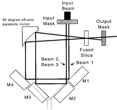
Fig. 1. TG FROG configuration. Beams 2 and 3 are vertically separated. M1 and M4 and M2 and M3 form two pairs of retro-reflectors with the inner pair (M2 and M3) on a motorized translation stage.
