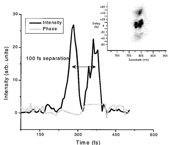
Fig. 6. FROG trace of a pair of near-transform-limited pulses separated by 100 fs along with its retrieved intensity and phase in the time domain.
