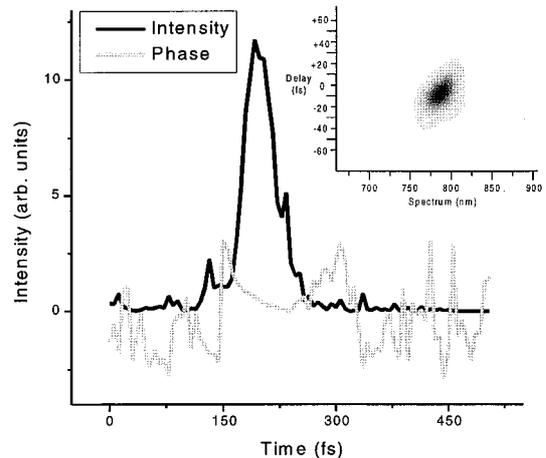
Fig. 5. FROG trace of a linearly chirped pulse along with its retrieved intensity and phase in the time domain showing a pulse duration of 50 fs.
