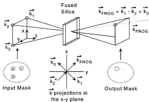
Fig. 2. Input and output mask specifications for DFWM. The  $\mathbf{k}_i$  vector corresponds to the  $i$ th beam. The input beam is 10 mm  $\times$  8 mm and the input mask holes are 1 mm in diameter with a 2-mm center-to-center separation. The output mask hole is 1 mm in diameter and is positioned at the image plane of the input mask.
