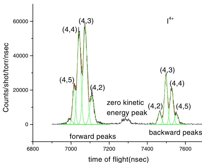
**Figure 2.** Typical TOF spectrum.
