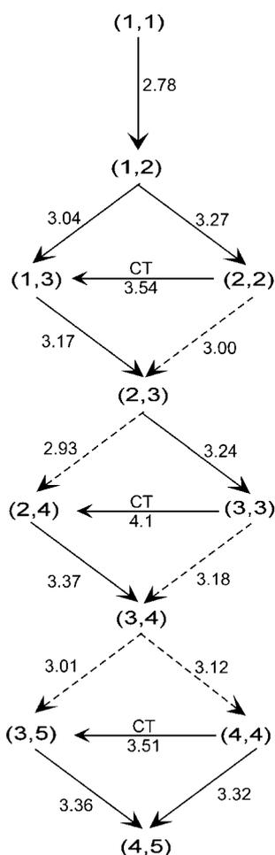
**Figure 4.** One-electron ionization pathways in molecular iodine. Numbers above arrows indicate  $R$  (ångstroms) at ionization. CT = charge transfer. Full arrows are allowed configurations whereas the broken arrows are unphysical (see figure 3 for error bars).
