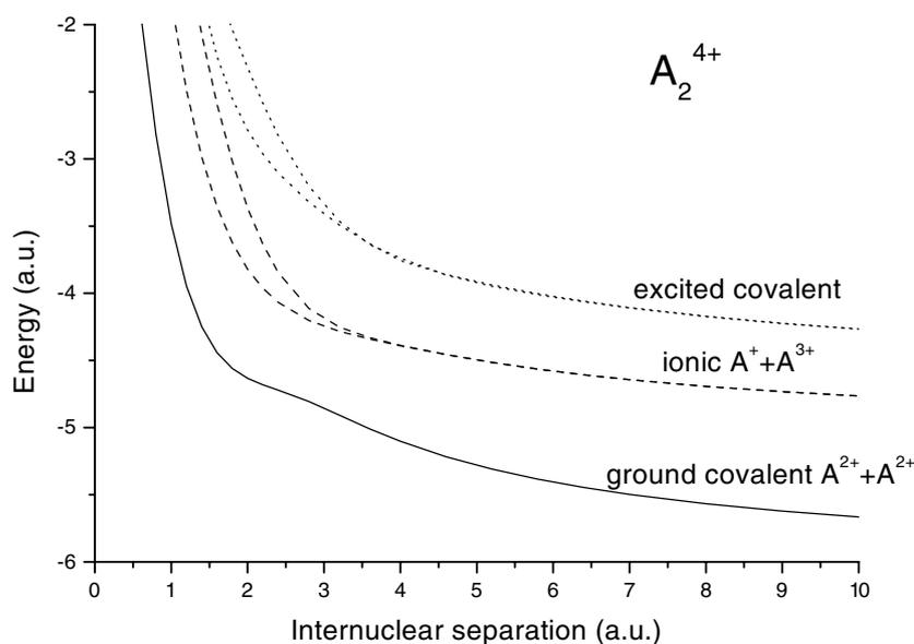
**Figure 7.** Covalent and ionic PE curves of a 1D molecule calculated using the procedure (see footnote 3). The ground covalent state of the molecule is represented by the full curve, the lowest lying ionic states by the broken curves and the excited covalent states by the dotted curves.
