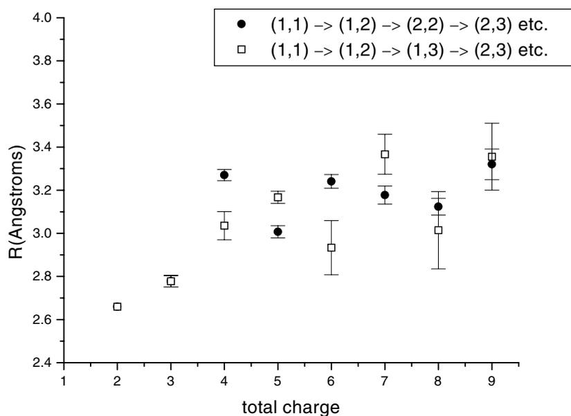
**Figure 3.** Internuclear separation at ionization (one-electron) for the symmetric and asymmetric pathways as a function of the total charge on the molecule. Error bars in our data reflect the uncertainty in  $\Delta t$  (see equation (4)) determined by fitting the various peaks in the TOF spectrum (see figure 2, for example).
