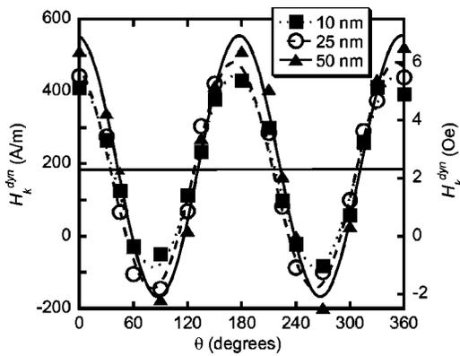
FIG. 3. The dependence of  $H_k^{\text{dyn}}$  on  $\theta$  for different thicknesses of Cu-capped Permalloy films is displayed. Uncapped Permalloy films showed no substantial differences. The lines are the fitted curves to the equation  $H_k^{\text{dyn}} = H_k^{(2)} \cos 2\theta + H_k^{(0)}$ . The solid line corresponds to the average value of  $H_k^{(0)}$  for all three samples.
