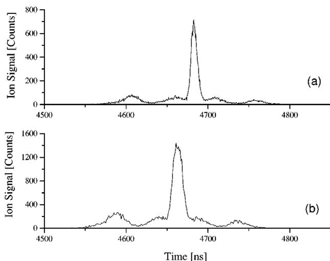
FIG. 3. (a) Normal time-of-flight (TOF) spectrum of  $N^+$ . (b) Time convolution of the TOF spectrum of  $N^+$ . The flight time of  $N^+$  in this figure is different from Fig. 2 because different TOF spectrometer voltages are used.
